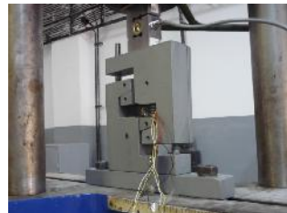
Figure 1: Shearing tests with Iosipescu Fixture System
