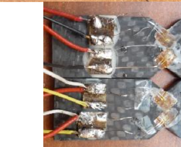
Figure 2: Specimen for shearing characteristics determination
