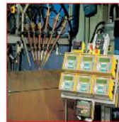
Multiple wires SAW: (six wires - same welding pool)
