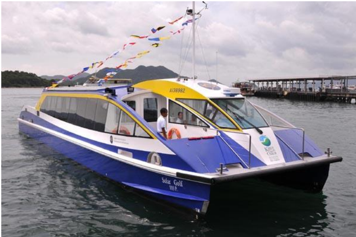
http://earthtechling.com Solar Water Ferry, Hong Kong, hybrid engine catamaran Solar Sailor Holdings
